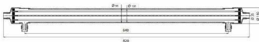
(Schematic of 4" dia - 3 m 2 membrane area - HF UF Cartridge; only for reference purpose)
